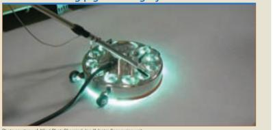
Photo courtesy of Allied PhotoChemical, Inc./Adastra floor curing unit
